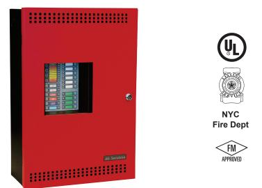
Secutron's MR-2320-R is a field configurable releasing control panel designed specifically for suppressing fires in high-risk environments. Intended for use with deluge sprinkler systems, pre-action sprinkler systems and agent release systems, the MR-2320-R controls the release of water or fire extinguishing agents in high-risk areas to prevent fast-spreading fires, minimize the need for costly equipment replacement and prevent detrimental business disruptions.
