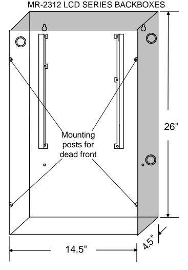
Place dead front over the backbox and electronics. Use the four #6 screws provided to screw the front to the backbox on the mounting posts as shown.
