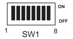
DIP switches are for assigning an address to the RAXN-LCD. Binary addresses 33 to 39 are available with the least significant bit being switch SW1-1 on the left and the most significant bit being SW1-6. The ON setting is active binary. DIP switches SW1-7 and SW1-8 are not used.
