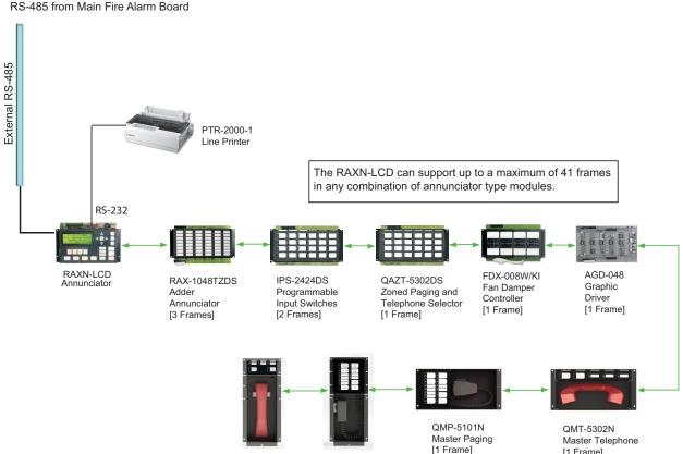
**QMT-5302NV OMP-5101NV** Master Telephone Master Paging [1 Frame] [1 Frame]
