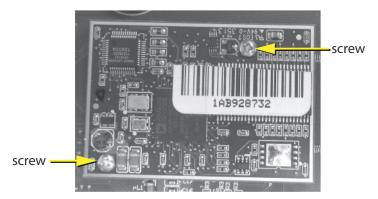
2. Gently wiggle the old core board (pull one side and then the other in a repetitive motion) until it is free of its connectors.
