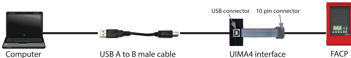
Figure 23 UIMA4 to P5 on main board
