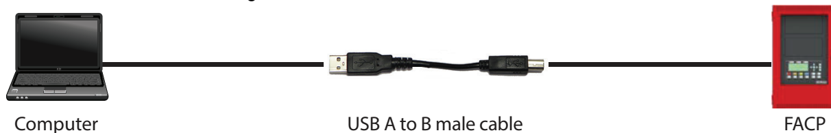
Figure 22 USB A to B plug cable to P13 on main board
