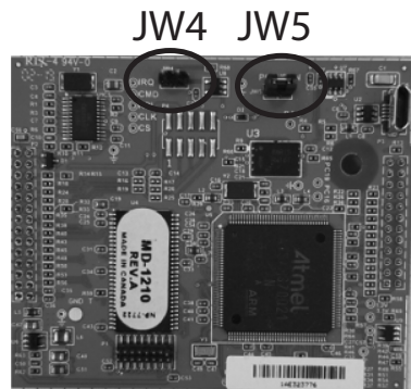
Figure 88 Jumpers on the MR-400 and MR-401 core board
