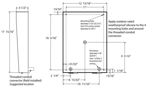
**Notes:** MMX-BB-1002WPA is a white model. MMX-BB-1002WPRA is a red model. Connect chassis ground stud to earth ground.
