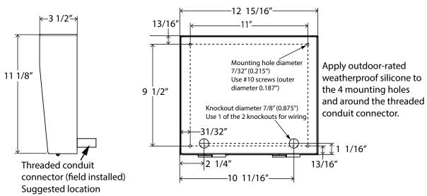
**Notes:** MMX-BB-1001WPA is a white model. MMX-BB-1001WPRA is a red model. Connect chassis ground stud to earth ground.
