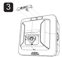
Secure the unit with the #4-40 x 3/8" screw and snap the nameplate over the screw.
