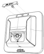
Attach the mounting plate to the box with 2 or 4 screws.
