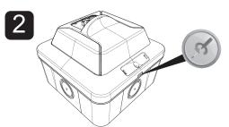
Insert a flathead screwdriver into the slot at the top of the unit and turn it to separate the unit from the mounting plate.
