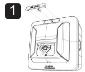
Remove the nameplate and the screw.
