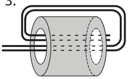
Wrap wire around and through Ferrite Bead until there are three loops as shown in step 4.
