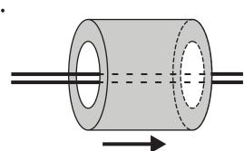
Thread wire through Ferrite Bead
