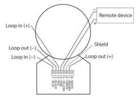
FIGURE 12: Loop wiring
