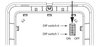
Device settings are located on the back of the unit to prevent tampering.
